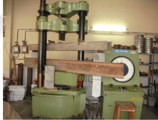
Fig. 1: Testing of ferrocement beam Channel section
