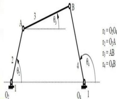
Fig. 1: Fourbar mechanism
